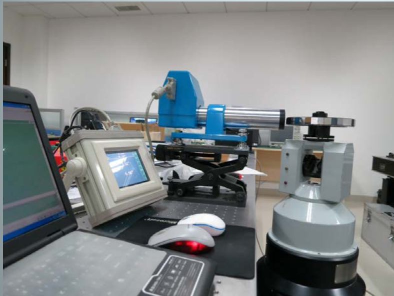
Horizontal Angle Calibration
