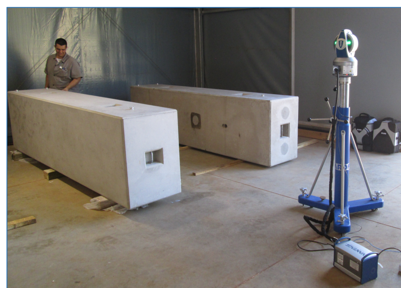
Concrete base geometry inspection
