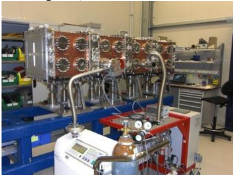
Figure 2 A supermodule of the RFQ in the assembly phase with the temporary isostatic supports and under vacuum tightness testing.
