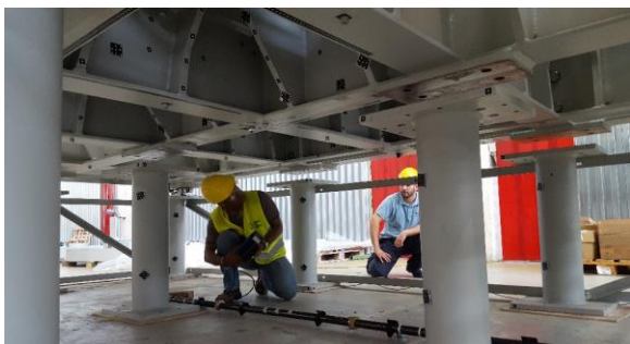
Figure 11 Survey with PG technique of ITER PS1 component for ITER project.
