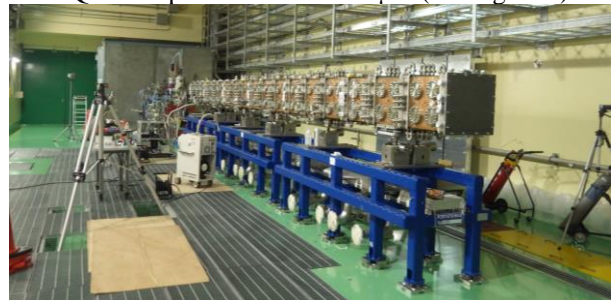
Figure 5 The RFQ after the alignment and connection of the three SMs.
