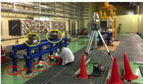
Figure 3 Alignment of the SM1 in the temporary position in the assembly hall.
