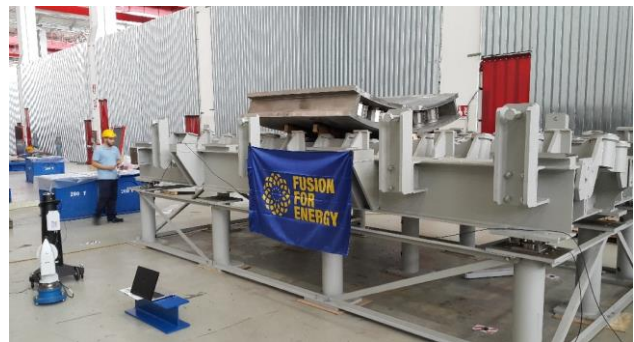
Figure 12 Laser tracker survey of the PS1 component for ITER project for comparison with PG.
