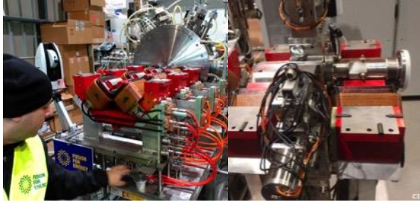
Figure 7 Top halves of the magnets disassembled (left) and installation of the scrapers, and beam pipe with BPMs (right).
