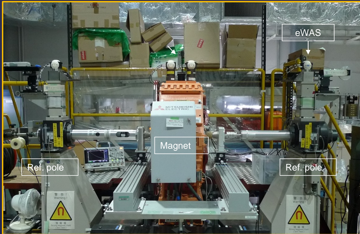
Wire alignment system for magnet fiducialization of magnet field measurement device.
