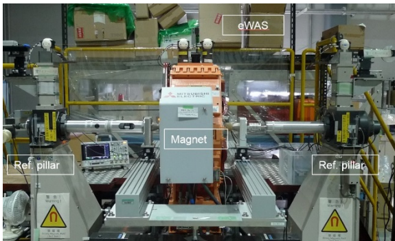
Figure 8: Wire alignment system for magnet fiducialization on the magnetic field measurement device.
