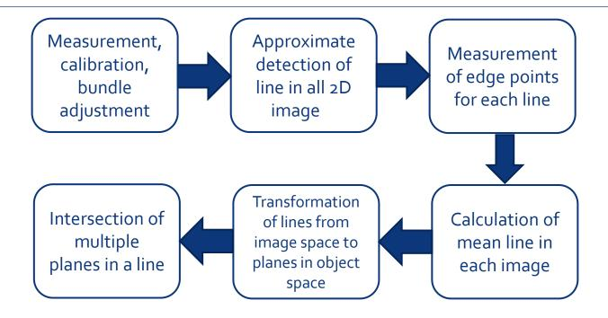
Line calculated by individual adjustment or within bundle adjustment
