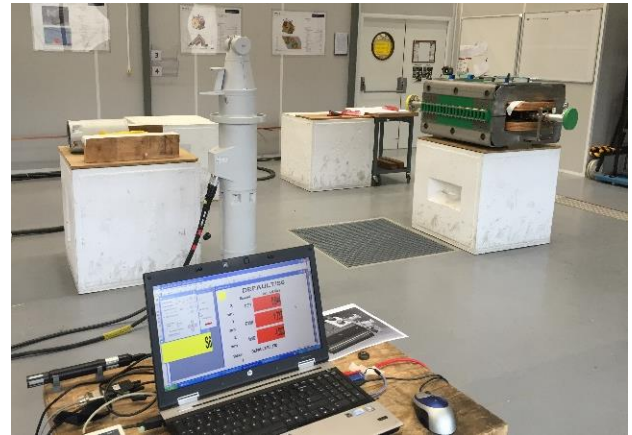
Figure 6 : vacuum chamber alignment in a horizontal bending with a LTD 500
