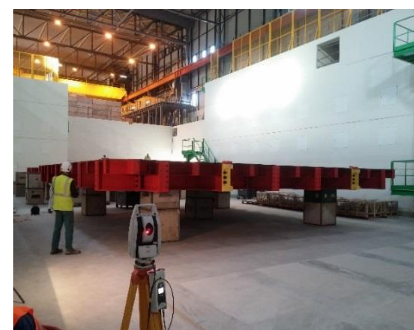
ProtoDUNE base supporting structure during shape control
