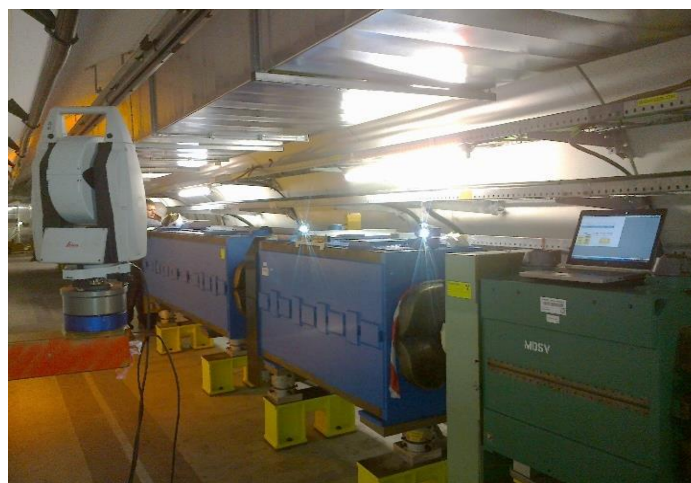
AWAKE : Alignment of magnet with Leica AT 401
