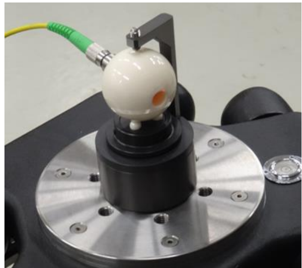
Figure 7. Prototype for localizing the FSI optical fibre tip consisting of a reference sphere and kinematic mount.
