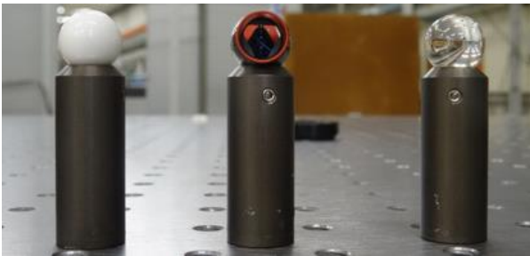
Figure 8: On the right is a 12.7 mm diameter TAFD55 glass retroreflector mounted on the same type of support as a Leica open air corner cube and a white ceramic micro-triangulation target of the same size.
