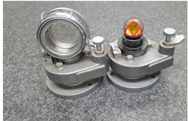
Figure 4: The 2 1/4" optical target (left) and the 1,5" CCR on a 2 1/4" adapter (right)
