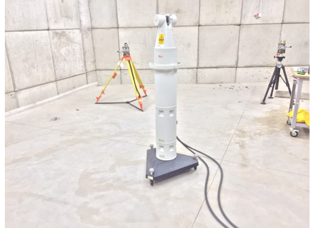
Figure 5: The xpr hall - step 6: measuring P4 and P5 by laser tracker
