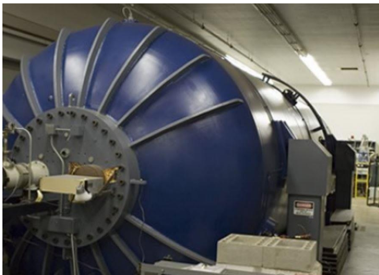
Figure 2. FN Tandem Van de Graaff accelerator University of Notre Dame, Indiana, USA.
