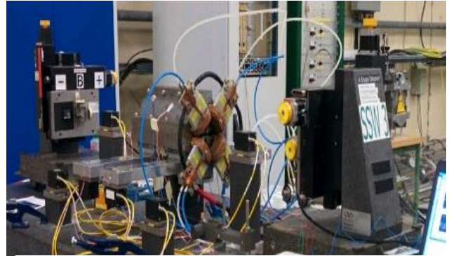
Figure 9: Measurement of magnet axis drift due to temperature setup
