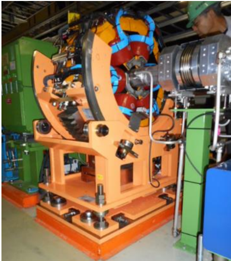
Figure 8: Sextupole magnet tilted by -30^\circ .
