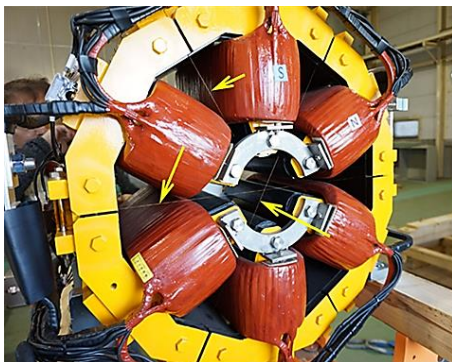
Figure 3: Crosshairs made by thin beryllium-copper wires stretched between opposite facing gaps of the pieces of the magnet return yoke. The positions of crosshairs are shown by yellow arrows.
