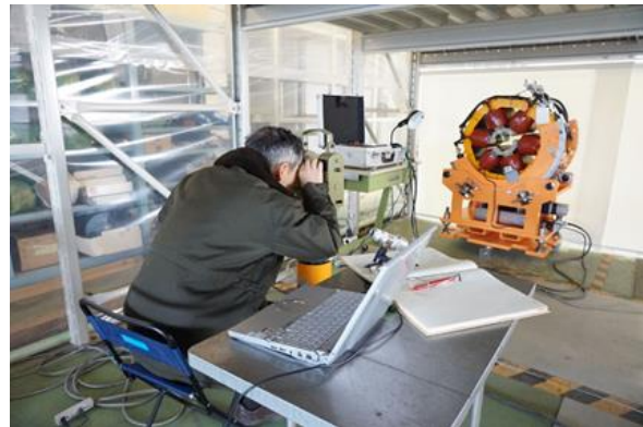
Figure 4: Measurement of the position of the near and far crossing points of the crosshairs with a theodolite.
