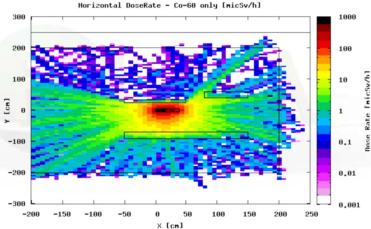
Filtering all isotopes but Co-60 (sensitivity to cobalt content in steel for long cooling times)
