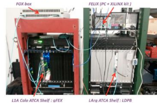
LATOME – Optical link tests with gFEX
