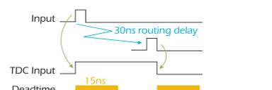
The falling edge of the input can not be detected due to the intrinsic dead-time of the TDC. Instead, routing is used to delay the falling edge until the TDC is ready again.
