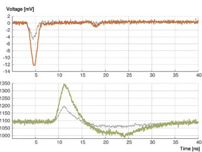
Example signals. Top: Input, Bottom: Output Shown are two typical PMT signals with 12 mV and 4 mV amplitude
