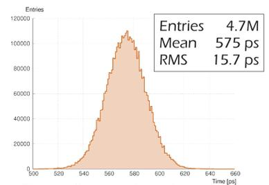
Timing difference between two channels of the same front-end module
