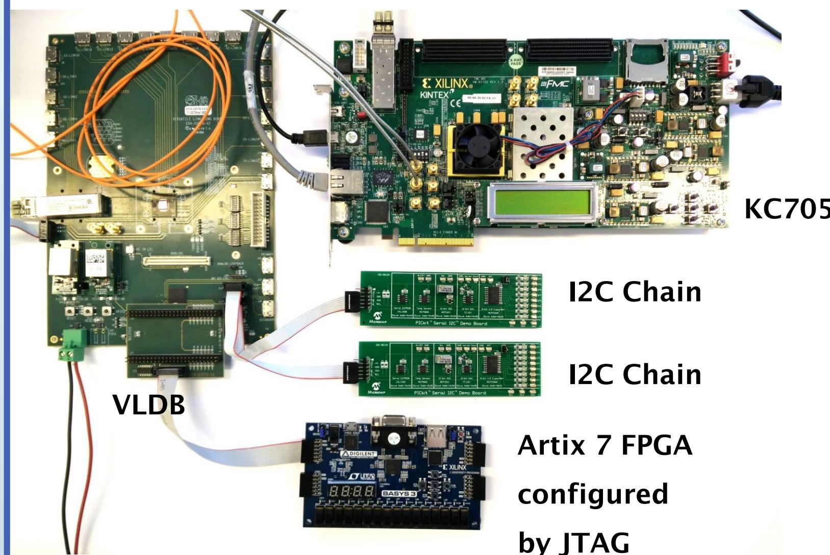
The picture above shows an example of SCA test setup\* which depicts two I<sup>2</sup>C demo boards and one FPGA used as slaves from the SCA. In this setup the KC705 sends data through the EC field of the GBT serial frame. The Artix 7 FPGA can be configured through the JTAG link controlled by the SCA.
