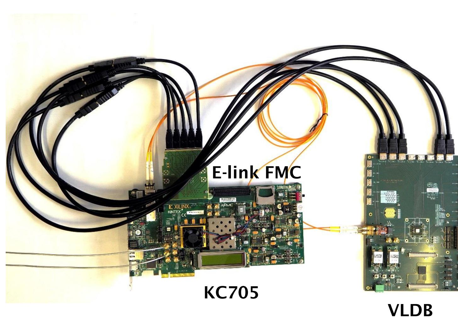
This picture shows a setup which consists of a VLDB, a KC705 board (acting as back-end board), an optical link and a 5 e-link connection through HDMI cables and an e-link FMC. In this way data can be serialized by the GBT-FPGA in the Kintex 7, transmitted over the optical link, recovered by the GBTx, distributed on the e-links and checked back in the FPGA.
