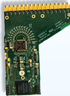
**SAMPIC** – The SAMPIC has 16 input channels with a sampling rate up to 10 Gs/s. Each channel works in a independent self-triggered mode and up to 64 sample can be acquired on each trigger. Such solution permits to sample the whole leading edge of the signal (~2 ns), allowing advanced offline reconstruction algorithms;
