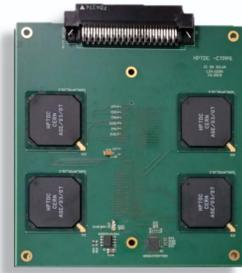
**HPTDC** – based on four HPTDC chips on the board which forms a token ring controlled by the SmartFusion2 FPGA on the readout board. Specially designed front-end board with four NINO chips 8 channels each is connected to the inputs of the HPTDC mezzanine;
