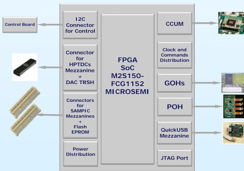
The main objectives of the board are to acquire on-detector data and trigger from the hybrids, to perform data conversion from electrical to optical format and to transfer it to the next level of the system. It also distributes the control information to the hybrids and collects different detector and board parameters.
