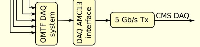
The OMTF DAQ is implemented together with the OMTF trigger algorithm [2] in the MTF7 MTCA board [3, 4]. The OMTF DAQ transmits to the CMS data acquisition system (CMS DAQ) the data, that were the source of the trigger decision, to monitor the trigger operation. Data from all detectors are concentrated, subjected to zero-suppression, and transmitted via AMC13 board located in the same MTCA crate.
