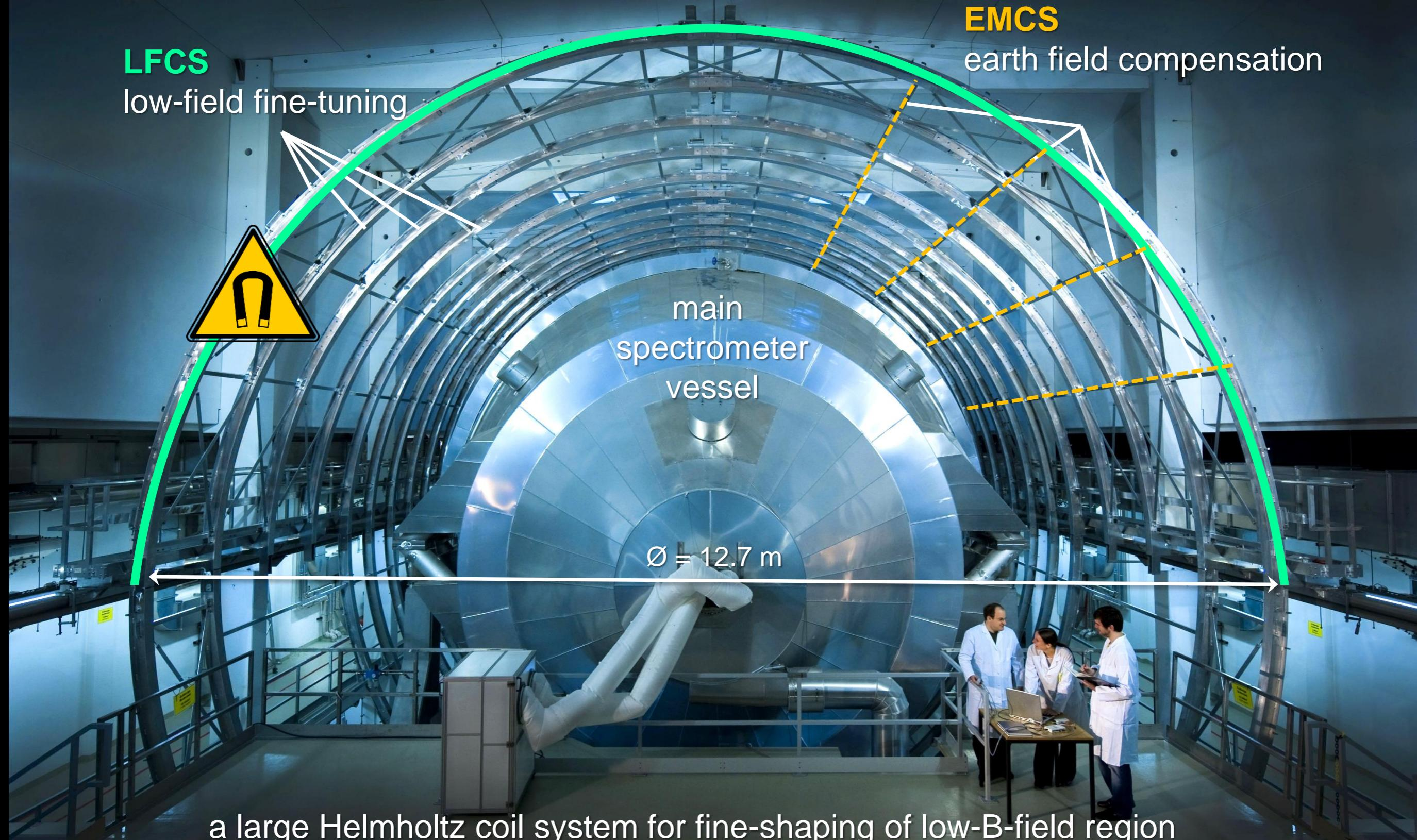
a large Helmholtz coil system for fine-shaping of low-B-field region
