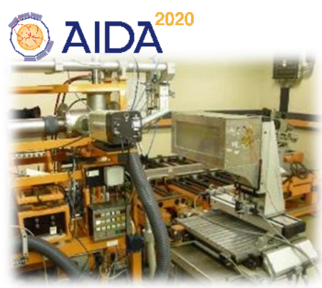
Device irradiation 23MeV protons and x-ray available on site
