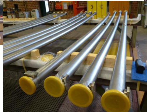
All dipole chambers delivered and shipped to GSI for NEG coating
