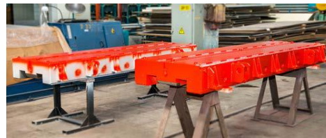
Second FOS magnet ready for assembly
