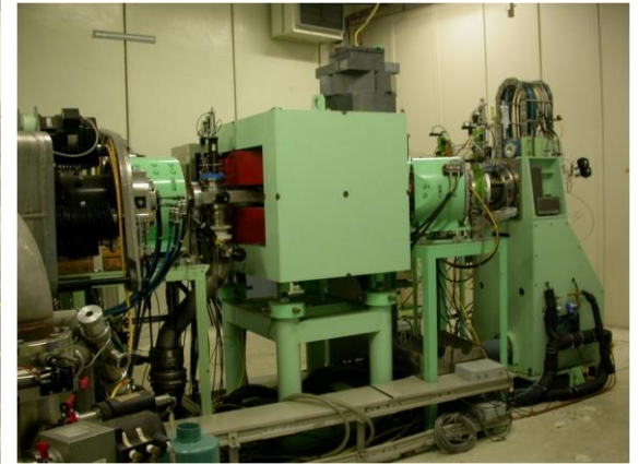
Positive ion machine with deflector (hot).
