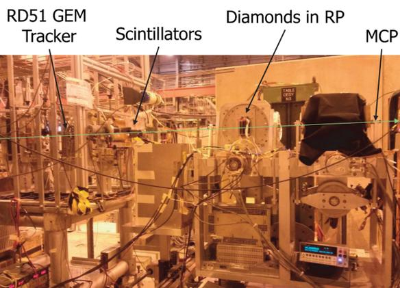
At SPS H8C test beam area we successfully tested diamond detectors' timing performance and efficiency inside a Roman Pot in their final settings (left).
