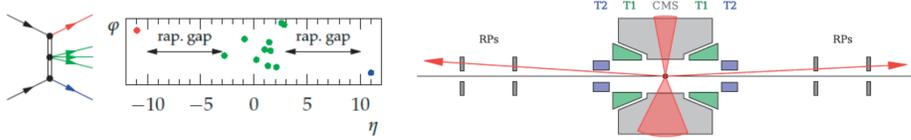
The installation of proton Time-Of-Flight (TOF) detectors in the TOTEM Roman Pots allows us to reconstruct the longitudinal vertex position and thus to assign the proton vertex to the proper one reconstructed by the CMS tracker, even in presence of event pileup.
