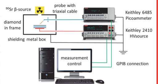
Computer controlled measurement setup was built to measure  $\sim$ pA leakage currents in pre- and final metallized diamonds with movable spring probe. Leakage current depends on crystal quality (e.g. impurity concentration) and metallization process.
