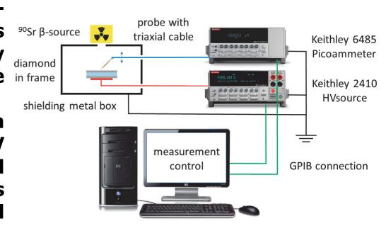
Computer controlled measurement setup was built to measure ~pA leakage currents in pre- and final metallized diamonds with movable spring probe. Leakage current depends on crystal quality (e.g. impurity concentration) and metallization process.
