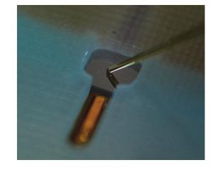
Bad diamond: high leakage current only at positive HV and unstable signal current only at negative HV
