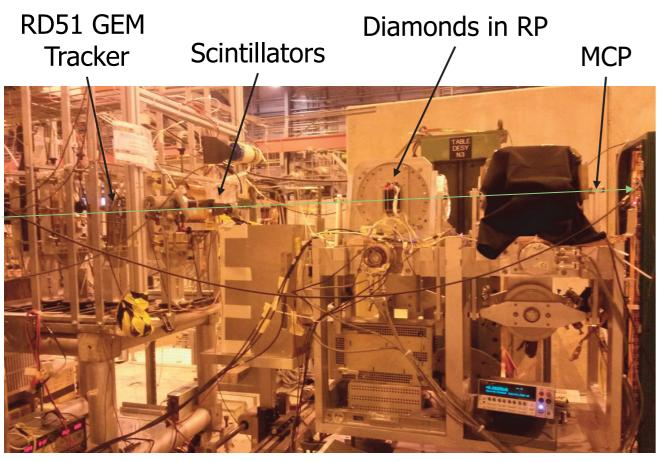
At SPS H8C test beam successfully area we tested diamond detectors' timing performance and efficiency inside a Roman Pot in their final settings (left).
