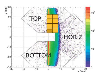
Track distribution in one RP in  $\beta$ \* = 90 m runs, for events with two protons in the final
