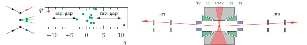
The installation of proton Time-Of-Flight (TOF) detectors in the TOTEM Roman Pots allows us to reconstruct the longitudinal vertex position and thus to assign the proton vertex to the proper one reconstructed by the CMS tracker, even in presence of event pileup.
