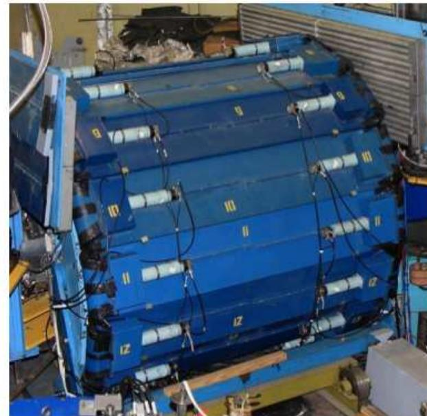
High-resolution NaI calorimeter with excellent tracking and PID
