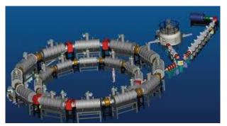
Design project for FFAG for radiotherapy. Still only a design - but got the UK accelerator community thinking about protons and light ions. Effects still being felt.
