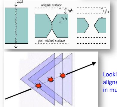
Looking for aligned etch pits in multiple sheets
