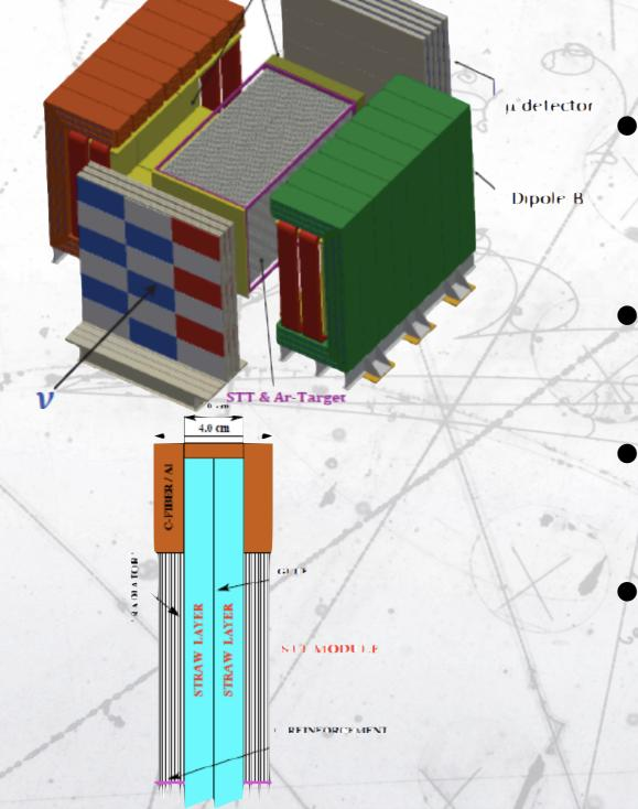
Magnetised (0.4T) high resolution straw tube design "a la" Nomad with plannar geometry.
