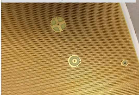
HV connections to the top and bottom LEM electrodes
