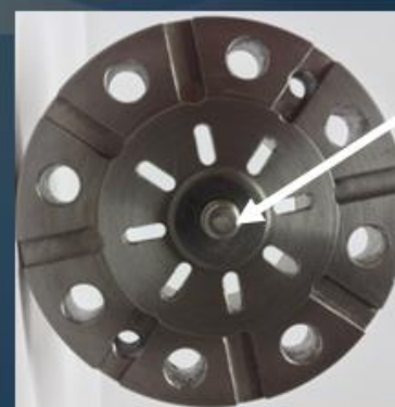
New plug with LHe channels
