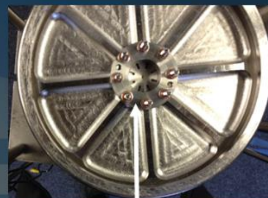
New plug with LHe channels
