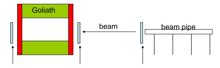
Proposed position for the 3 Trigger & tracking stations
