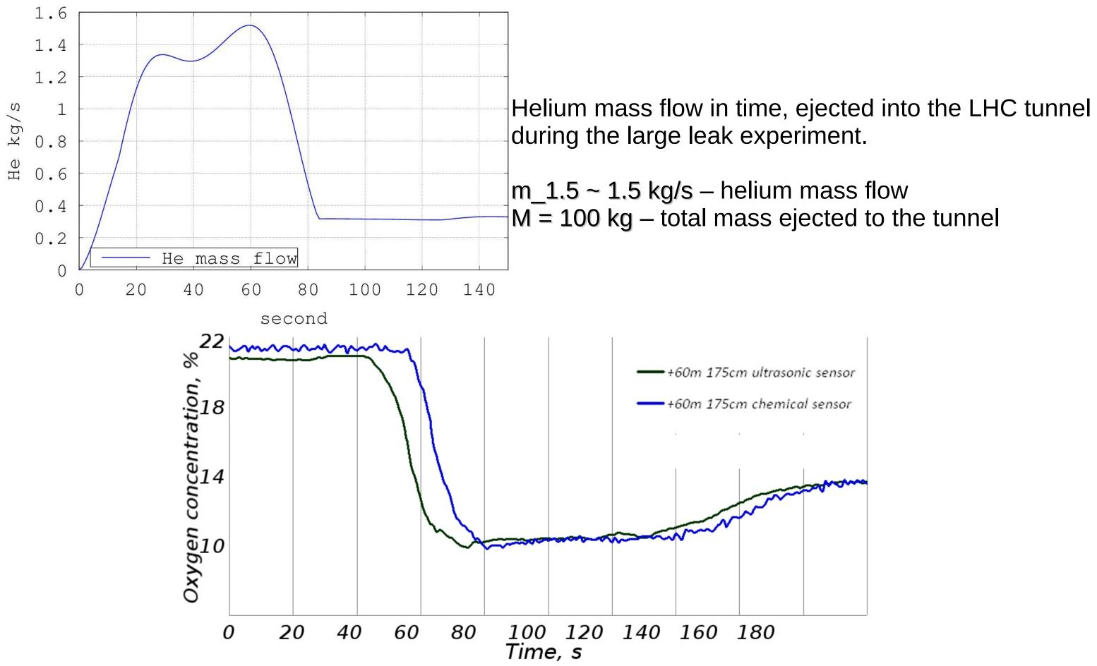
A comparison of dynamic oxygen content measurements produced by ultrasonic detector (black line) and electrochemical detector (blue line).
