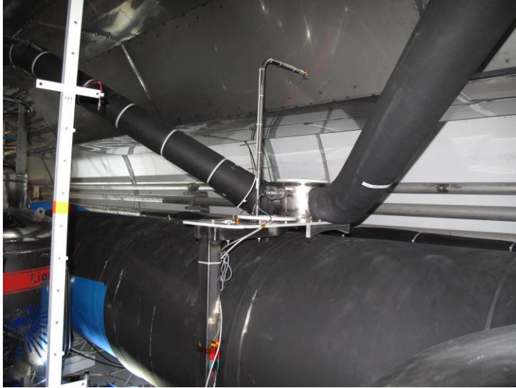
Helium dewars in place connected to the spill point. Dewars are pressurized by warm helium gas.
