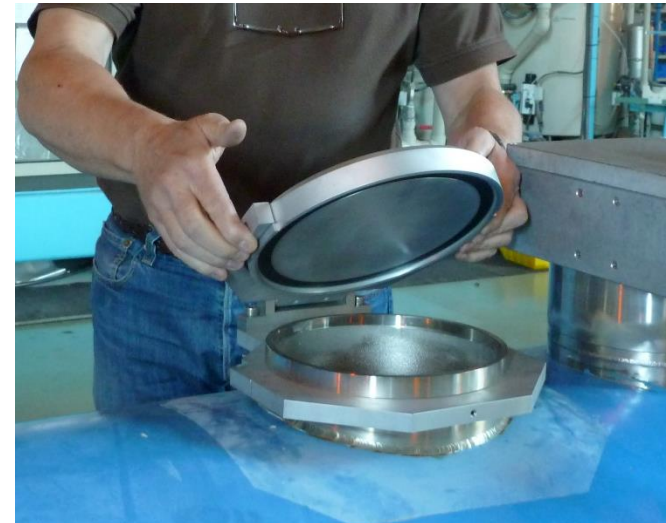
1 flap valve per sub-sector (opens first, can take up to 1 kg/s, re-closes)
