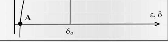
$$F_{\max} = \frac{C_a}{s_o^n} \left[ \left( \frac{m}{n} \right)^{\frac{-n}{m-n}} - \left( \frac{m}{n} \right)^{\frac{-m}{m-n}} \right]$$
