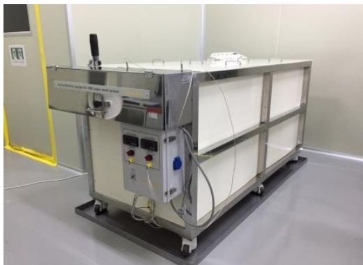
Etching/cleaning bath for Large GEMs
