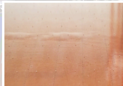
Bubbles on the resistive surface, caused by air enclosures between the PCB and the Kapton foil (left) and a series of folds in the foil.
