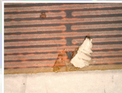
Two examples of contaminations: A piece/drop of metalized glue or silver printing paste (left), detergent remnants (right).
