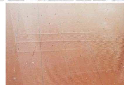
Bubbles on the resistive surface, caused by air enclosures between the PCB and the Kapton foil (left) and a series of folds in the foil.
