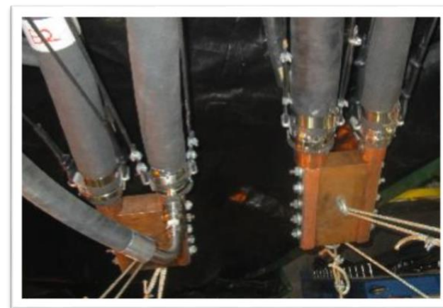
Cables: 24h Short Circuit Test
