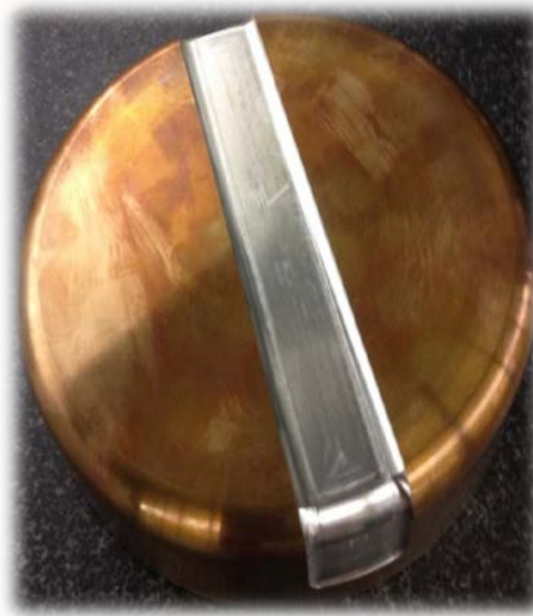
thin window \sim 300 \mu\text{m}
