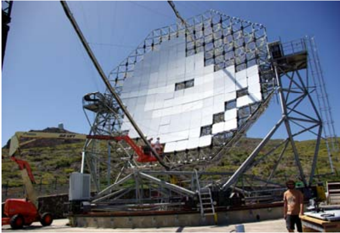
MAGIC telescope diamond cut metal mirrors
