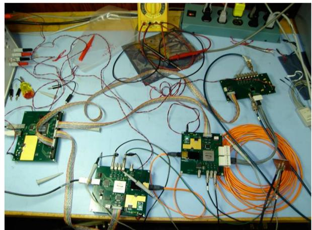
Figure 5: Test setup for the digital ADC logic.
