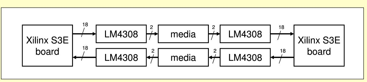
The LM4308 chip is an SLVS serdes, which can be hardwire-configured to be either a serializer or a deserializer. In the test, two LM4308 chips are serializers while the other two are deserializers.
