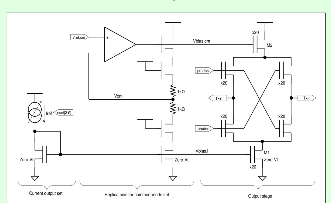
The transmitter is implemented by a Nover-N driver which the current steers given by the current source M1. The current is set by a 4-bit digital switch (not in the figure).
