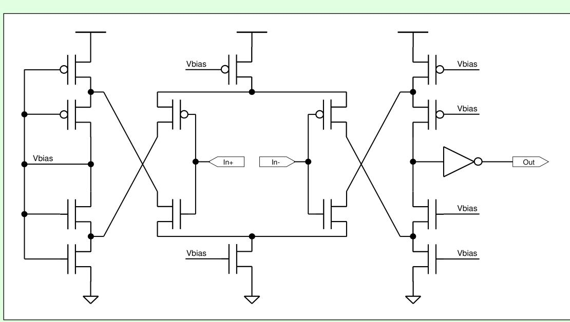
In power-down mode the biasing is switched off. This prevents toggling on the output. The receiver consumes 210 µW at 320 Mbps, 1.2V supply and with a 64 fF output load.
