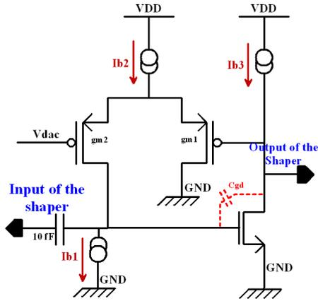
Figure 5: shaper schematic
