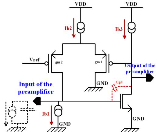
Figure 4: preamplifier schematic
