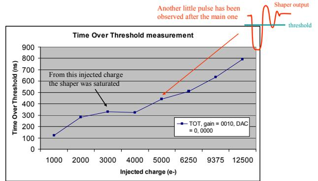
Figure 10: TOT for different injected charge values
