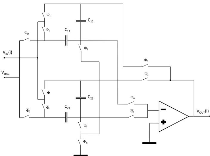
An important draw-back of the double sampling implementation is the introduction of a different timing skew between even and odd samples. This problem was overcome by the insertion of a synchronization switch that makes the sampling circuit skew insensitive.
