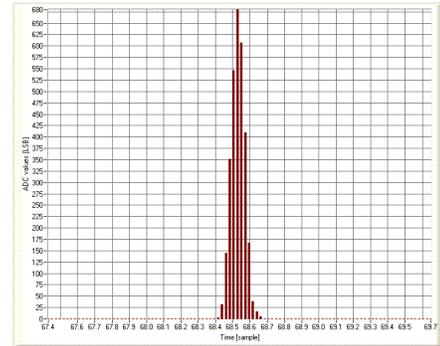
Figure 14: dual-pulse time difference distribution after correction.
