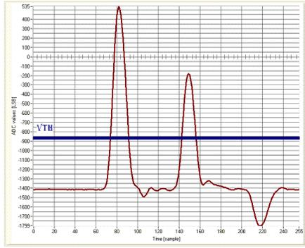
Figure 7: Two pulses generated by an open cable.
