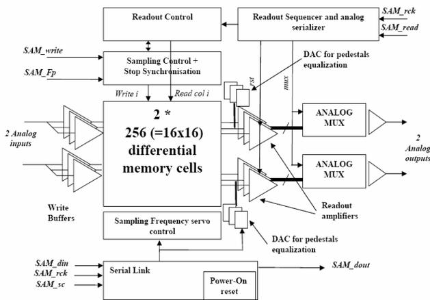
Figure 1: Block diagram of the SAM chip.
