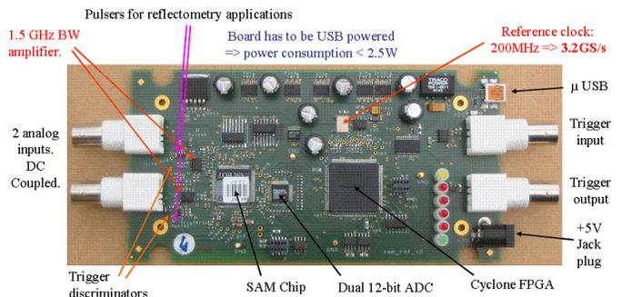
Figure 3: the USB Wave Catcher board
