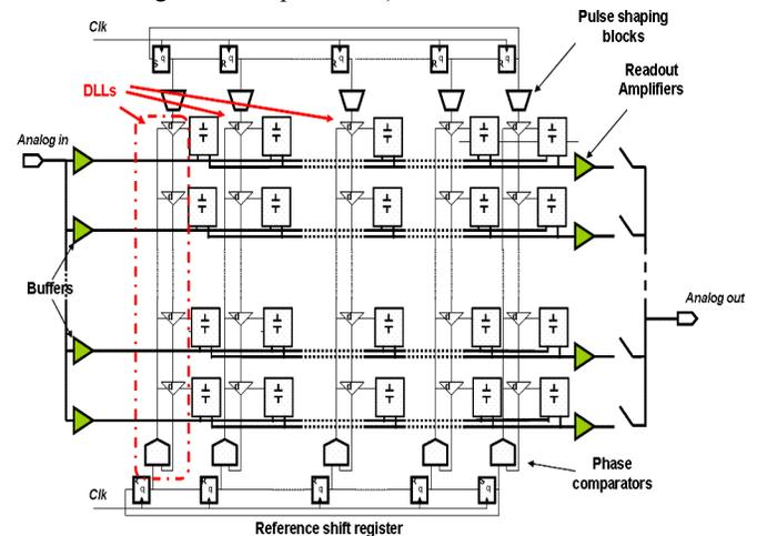
Figure 2: Principle of the sampling DLL matrix.
