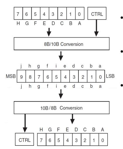
The 8B/10B coding is used by many protocols such as Fiber Channel, Gigabit Ethernet, PCIe and XAUI. The 8B/10B coding algorithm achieves: DC balanced data stream; Sufficient level transitions; Unique code groups Stratix II GX devices support two dedicated 8B/10B encoders in each transceiver channels. It works in cascade mode and complements the word aligner to achieve boundary synchronization.
