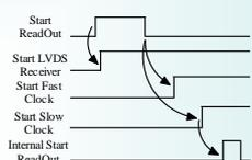
At the end of the readout, clocks and LVDS receivers are stopped synchronously. Effective PowerOn release is done after few clock ticks (2-3).
