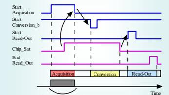
In neutrino experiment, acquisition is never stopped. This is the case for PARISROC chip which can handle an acquisition active all the time. During its conversion and readout phases, discriminated analog signals can be stored in the SCA if it is not full.
