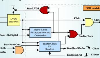
The POD module is divided in 3 parts. One is activated and managed by the DAQ during common phases: acquisition and conversion. The second one is set during the readout by the daisy chained token. The last one manages the LVDS receiver.
