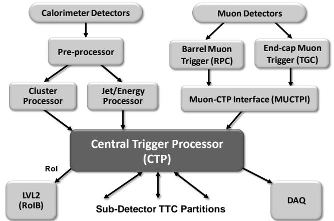
Figure 1: Overview of the ATLAS Level-1 Trigger
