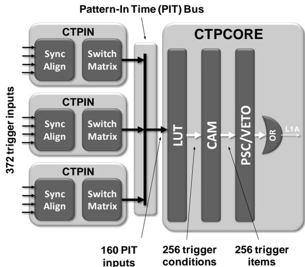
Figure 4: CTP trigger path
