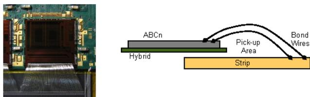
Figure 10: Bonding pattern of the ABCn chips
