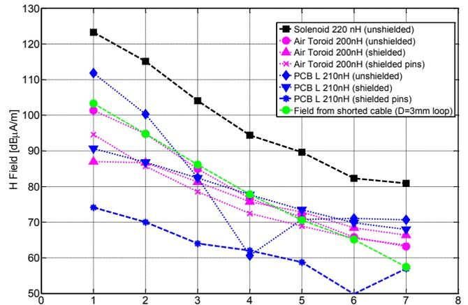
Figure 4: Magnetic field radiated by the inductors.
