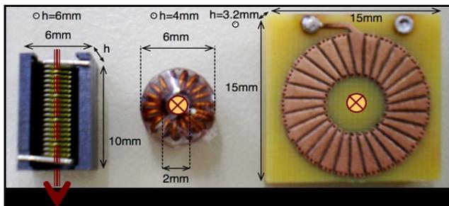
Figure 3: solenoid (left), air core toroid (center), PCB toroid (right).
